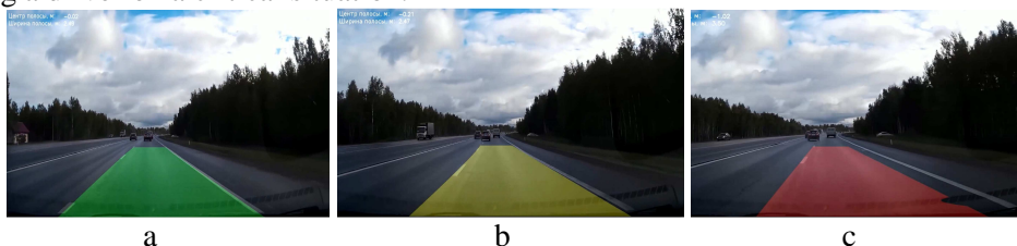
Figure 8. Visual road marking module: a – green zone, b – yellow zone (0.2-0.3 m deviation), c – red zone (over 0.3 m deviation)
