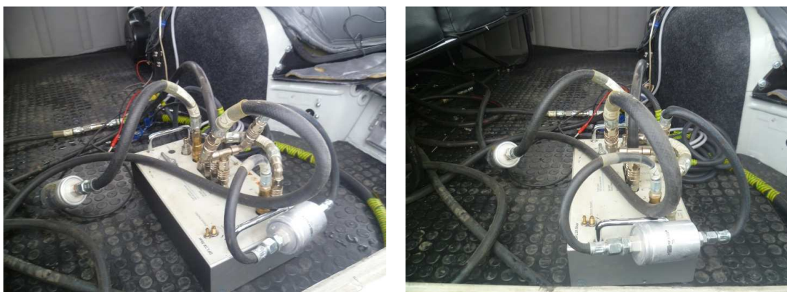
Figure 3. Installation of DFL3x flowmeter in a carburetor
