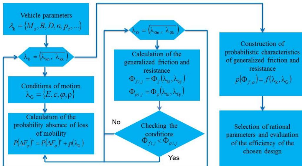
**Figure 3.** Block diagram of the methodology for evaluating the structural parameters of the chassis and efficiency criterion defining.
