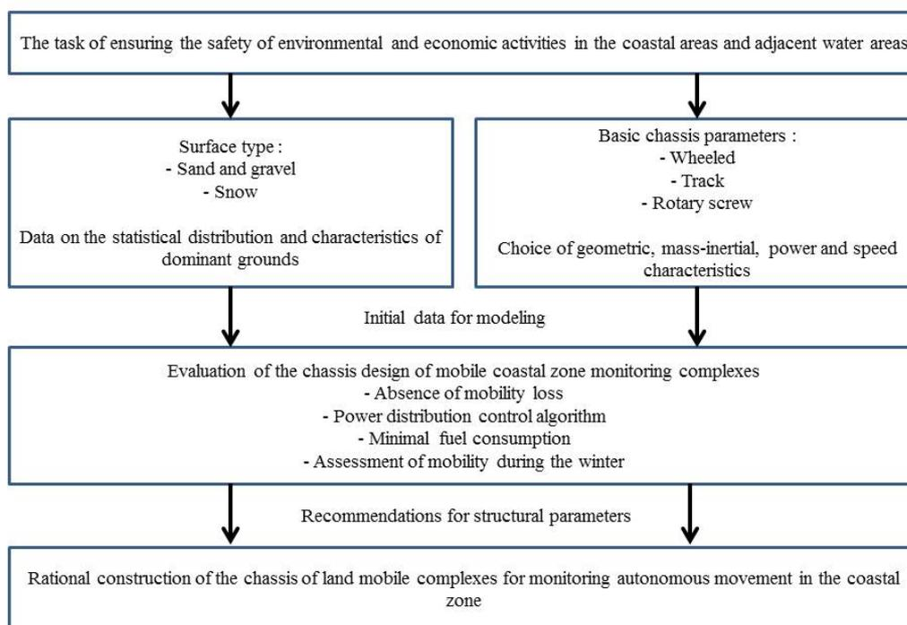
**Figure 4.** Block diagram of the method for designing the chassis of mobile monitoring sets.
