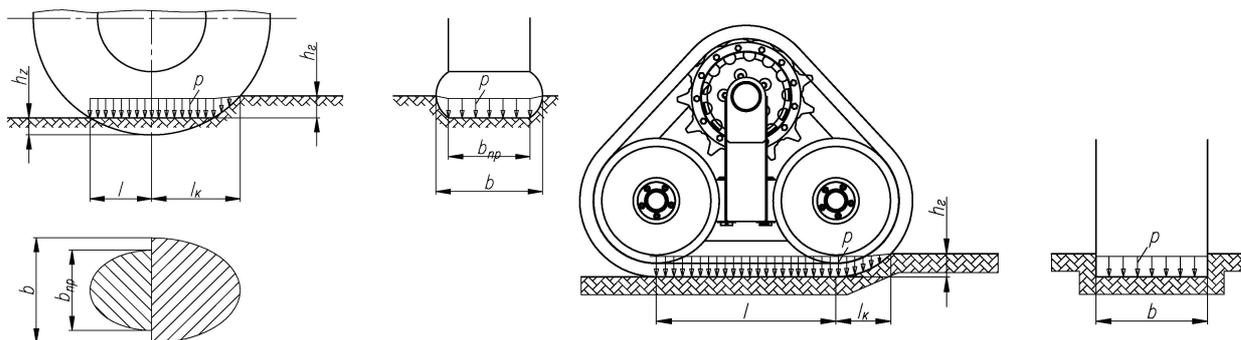
**Figure 2.** Design diagram of wheeled and track movers' interaction with soil.
